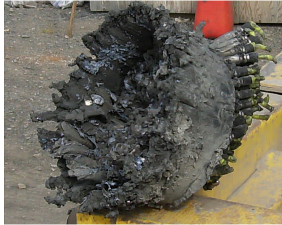
Cluster of detonated caps fused together
