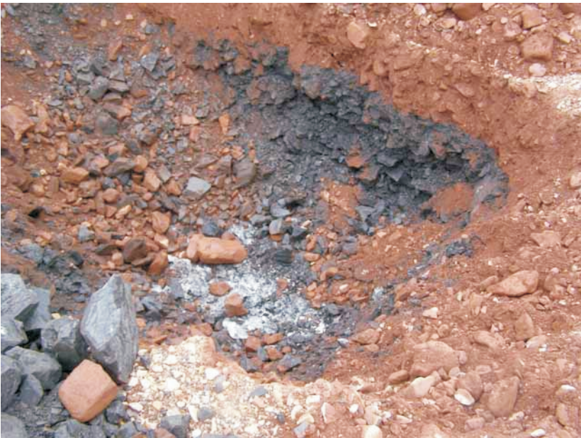
Photo 28 Test pit excavated through Test Cell cover. Note ice in shale at bottom of test pit.
