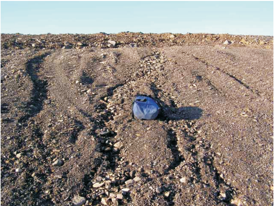
Photo 52 Minor rill erosion in southwest corner of Oceanview Open Pit cover. Note self armouring occurring.
