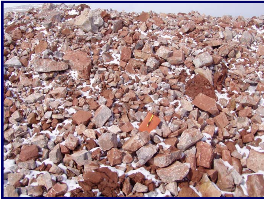
Photo 5 May 20, 2005 Stockpile of Type 2 riprap. Note field book for scale. Also note red staining on surface of rock.
