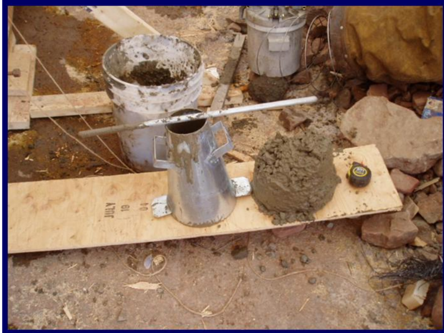
Photo 22 - September 29, 2005 Slump test from concrete used in the cut-off wall.
