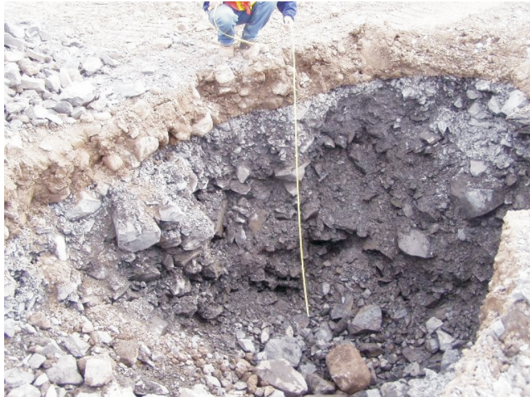
June 22, 2005 K-Baseline Portal Cover thickness test pit. Note particle size distribution of shale file.
