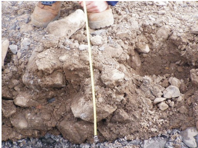
June 22, 2005 K-Baseline Portal cover thickness test pit. Note particle size distribution and thickness of armour material.
