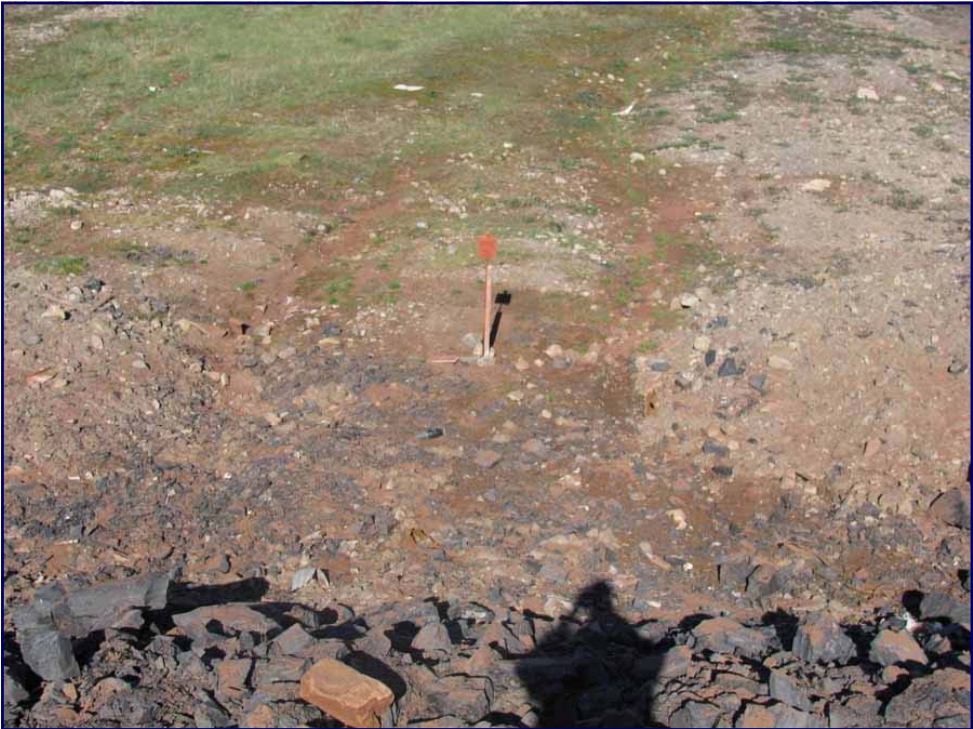
Photo 36 Seepage water monitoring station at toe of the landfill cover. Note no water is running here.
