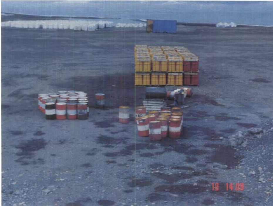
Photo # 8 Ground contaminated with waste oil at waste oil storage and consolidation area. Open oil tray in centre of photo.
