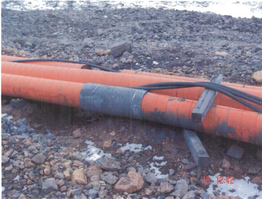
Photo #1 Tailings conveyance line flange, cause of spill 02-260.
