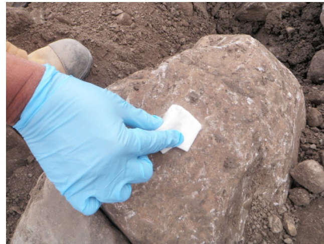
Photo 16: Collecting a swab sample from the surface of a rock that had been screened (August 30, 2012)
