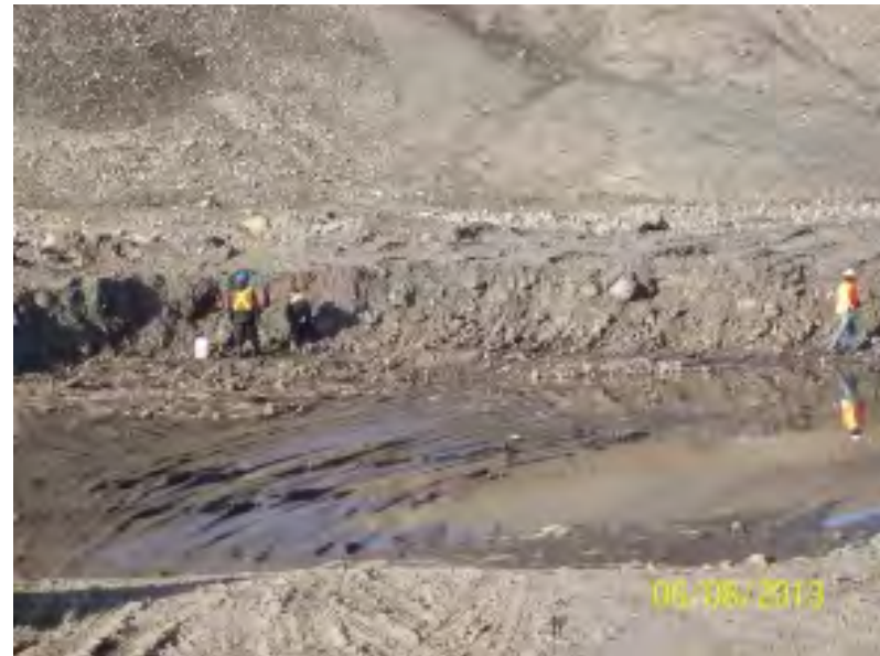
Photo 4: Samples were collected along the walls and at the base of the excavation at Area 4.
