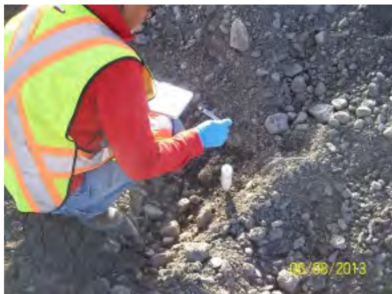
Photo 19: Moisture monitoring the biopiles.
