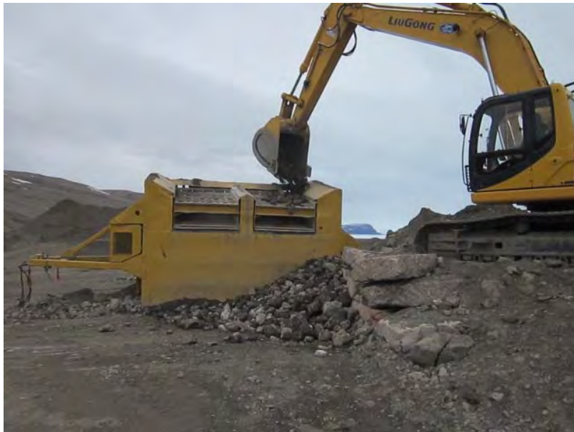
Photo 5: Rock rejected by vibrating screener.
