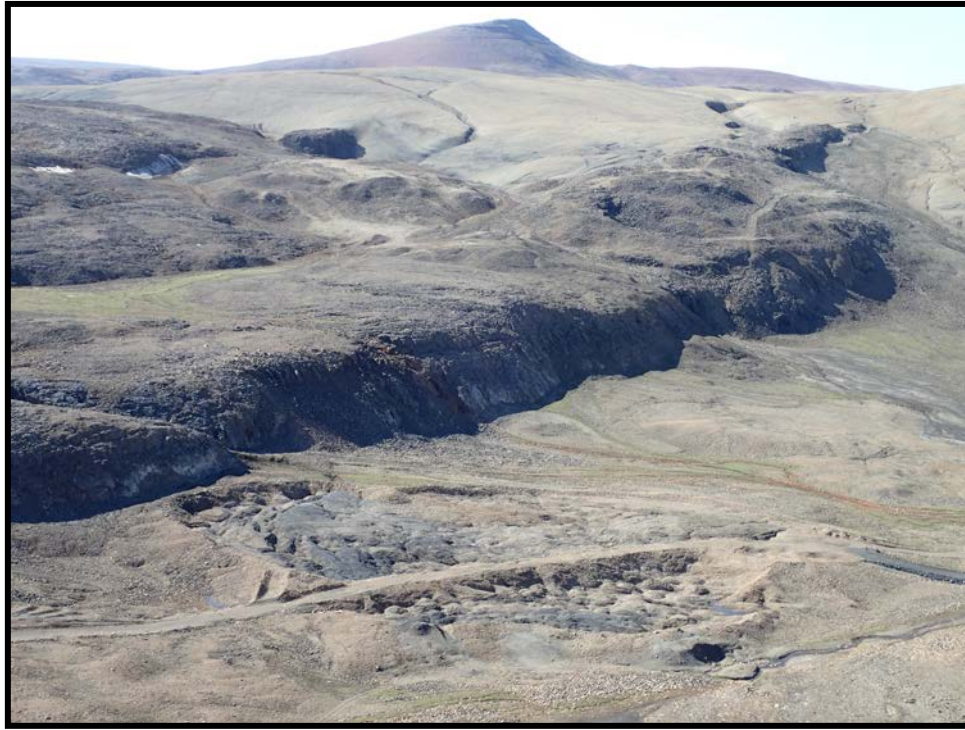
Photo 79. Kuhulu Lake Road Armour Quarry—Thermokarsting in floor of quarry. Note minor ponding near northwest corner.
