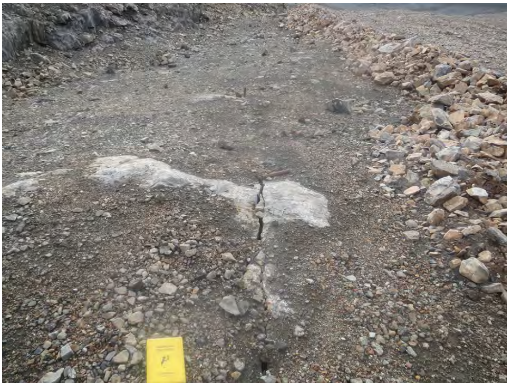
Photo 38. West Open Pit—Crack in crown pillar. No visual change in the 10 years since closure.
