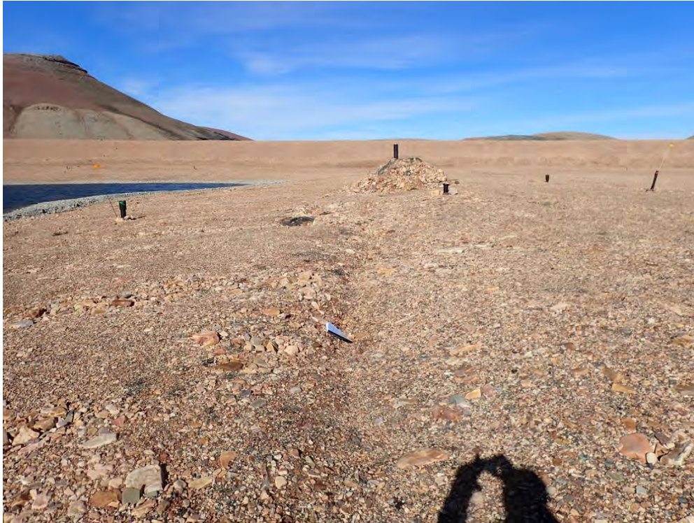
Photo 23. Test Cell—Settlement trough along edge of East/West Test Cell dike.
