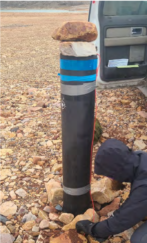
Photo 38. Test Cell Cover System – Thermistor datalogger installed at instrument BGC05-04.
