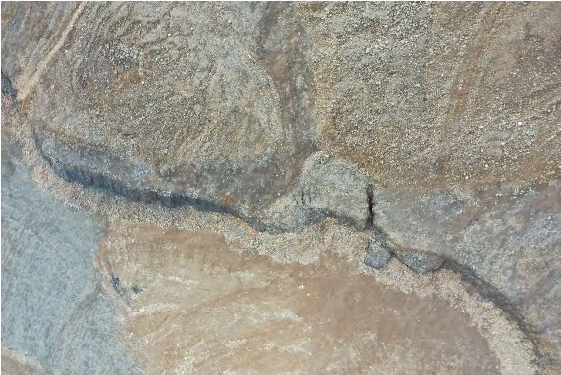
Photo 53. East Open Pit - Cracking in crown pillar, as seen from UAV.
