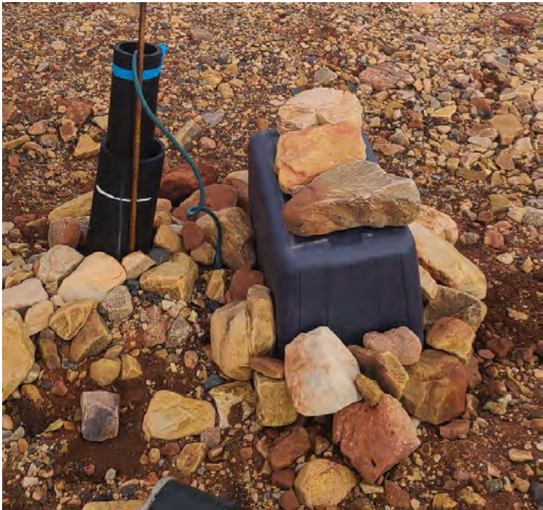
Photo 25. West Twin Dyke – Thermistor datalogger installed at instrument BGC05-15, after weatherproofing.
