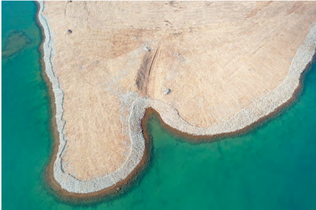
Photo 34. Test Cell Cover System – Breach in Test Cell Dyke as seen from UAV.
