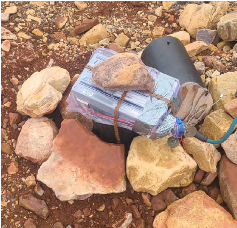
Photo 24. West Twin Dyke – Thermistor datalogger installed at instrument BGC05-15, prior to weatherproofing.
