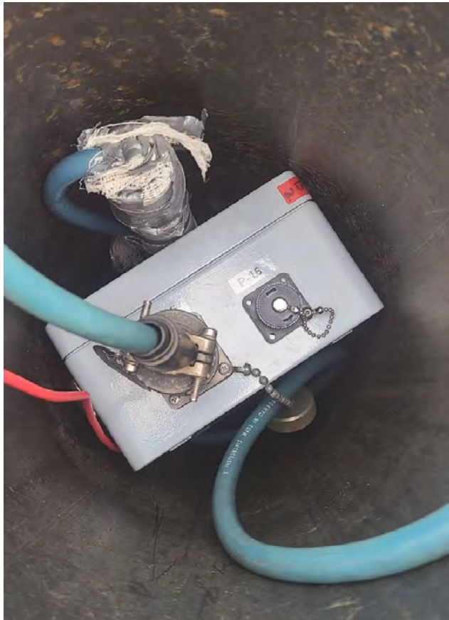
Photo 37. Test Cell Cover System – Thermistor datalogger placed inside protective casing at instrument BGC05-04.
