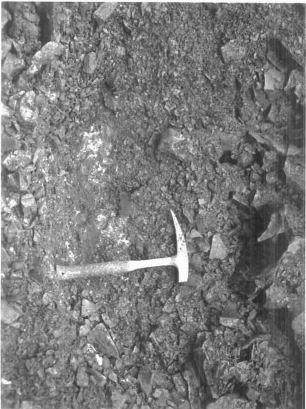
26-Jul-04 Photo 046 Area 14 Ice bonded shale in the bottom of Test Pit #2.
