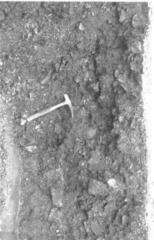
26-Jul-04 Photo 040 Area 14 Side wall of Test Pit #1. Note geological hammer for scale. Also note grain size distribution of shale which was observed to be coarser than the shale observed in test pits excavated in Test Cell Test Cover #1.
