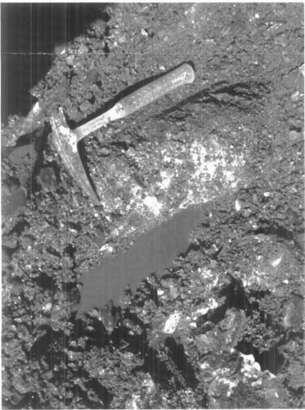
22-Jul-04 Photo 025 WTDA View of ice-saturated layer at base of Test Pit #4 in Test Cell #1.
