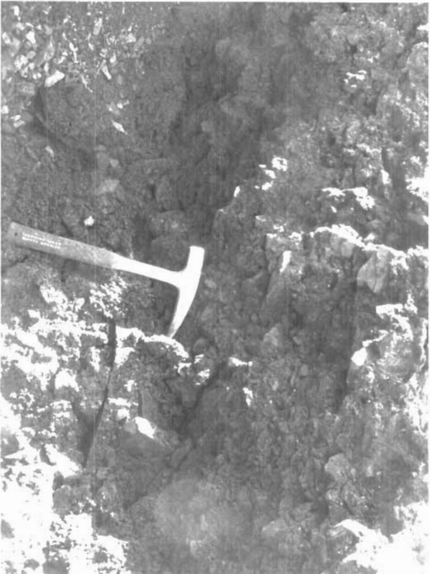
22-Jul-04 Photo 024 WTDA View of side wall of Test Pit #4. Note grain size distribution of shale including cobbles, gravel, sand and silt.
