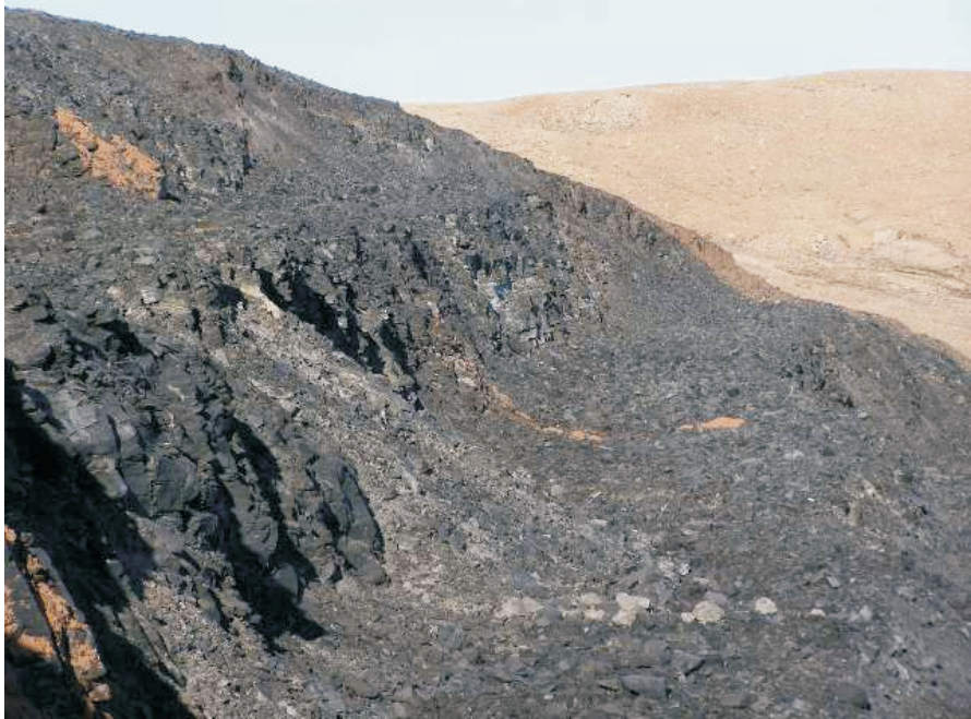
Photo 69 Benches in Mt. Fuji borrow area. Note ravelling occurring onto benches creating a sloping surface.
