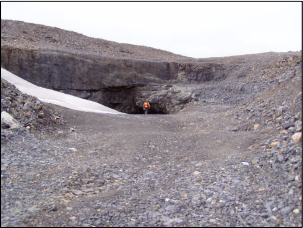
VIEW OF EAST TRENCH (JULY 2004). NOTE: MUCH OF THE TRENCH HAS ALREADY BEEN INFILLED WITH WASTE ROCK.
