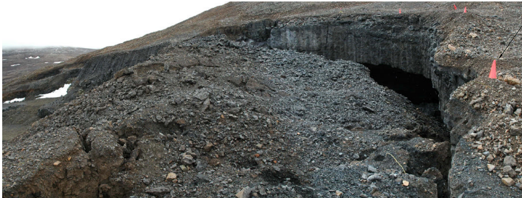
PHOTO 1 (SEPTEMBER 2004) TAKEN FROM NEAR PILON 1 LOOKING SOUTHWEST. VIEW OF PILE OF BLOCKY DEBRIS FROM HORSESHOE BLAST AND OPENING INTO 38-11 STOPE.
