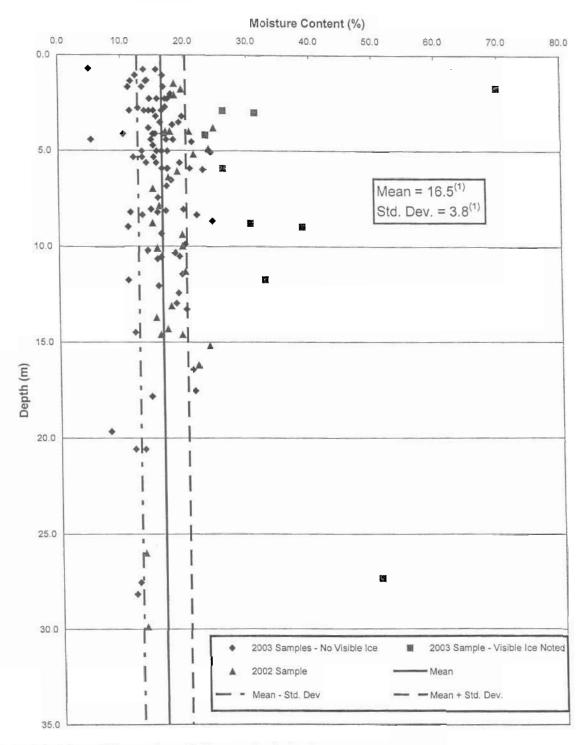
Note: (1) Calculated from 108 samples of tailings collected in 2002 and 2003 in Surface Cell and Test Cell Dike and toe of WT Dike containing no visible ice.
