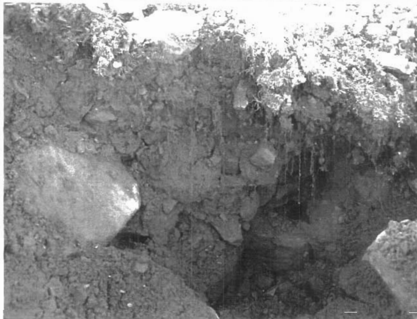
Photo of sidewall of test pit from spillway area investigation in 2002. Note variety of grain sizes.
