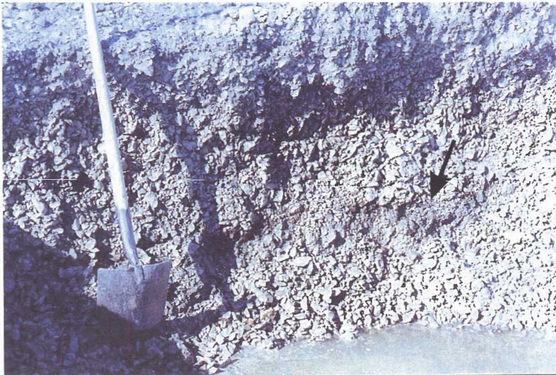
Oil stained layer evident at depth. (TP 91 at 0.5m, oil bladder spill area).
