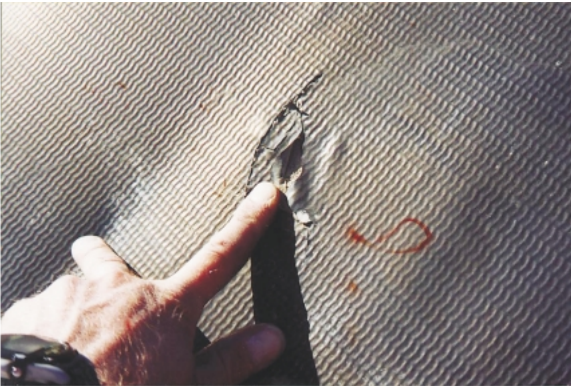
Partial surficial tear in tank farm liner on internal face of north limb of perimeter containment dyke, August 1, 2000.
