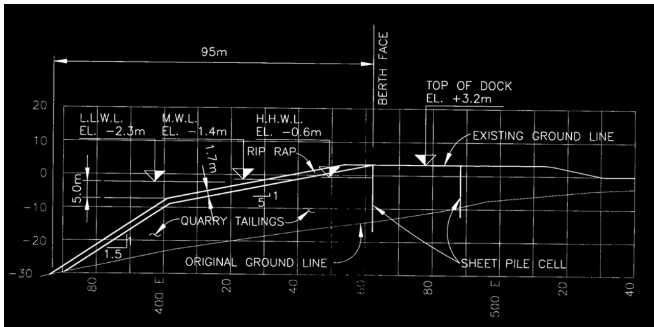
Figure 9: Cross-section through dock at Station 1400 N
