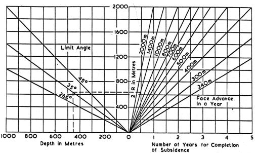
Fig. 33 Nomogram for estimating duration of subsidence.
