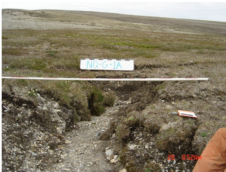
At waypoint NQG1A depth of erosion gully is 72 cm. Signboard has top bars at 10 cm intervals.
