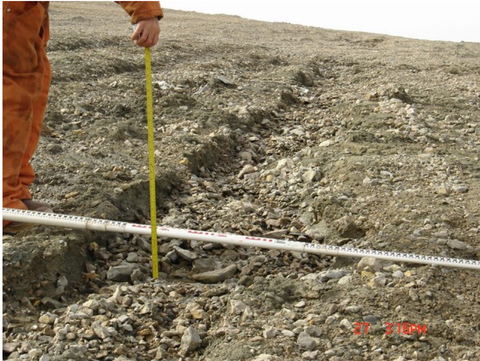
Erosion gully at waypoint OLF GUL1 has a depth of 20 cm.
