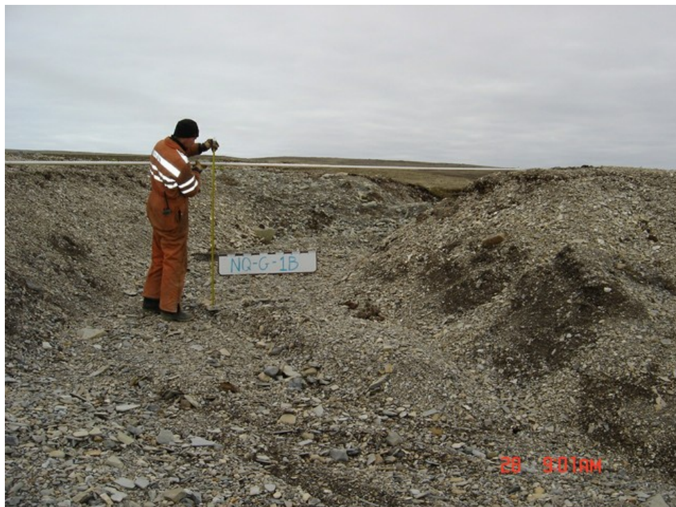
At waypoint NQG1B, depth of gully is 1.4 m, and width is 5.6m at base.
