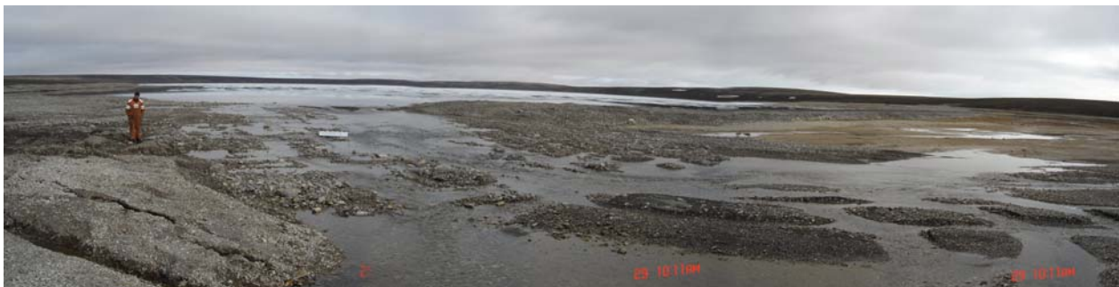
View north and east from waypoint GLWB2 looks upstream at outlet channel with wave break structure extending to the right. Material in channel is gravel sized and flow is only slightly turbid. Water quality sampling indicates that turbidity levels downstream at the main dam were low, evidenced by TSS measurements of 3 mg/l, at or below detection, on July 24 and July 31 st 2005.
