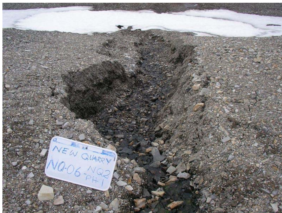
2006 – Close-up view of erosion gully at waypoint NQ2 PH1, showing relatively small width, and apparent tendency to be self-armouring, with no apparent changes from 2005.
