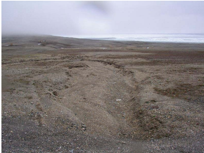
2006 – View to northwest at waypoint NQGTOP1 of a thaw/erosion gully on slope between road to Frustration Lake and the new Quarry area. This feature extends down to the top of the fan shown in photographs taken from waypoint NQ6 (see below). No discernible change since 2005 inspection.
