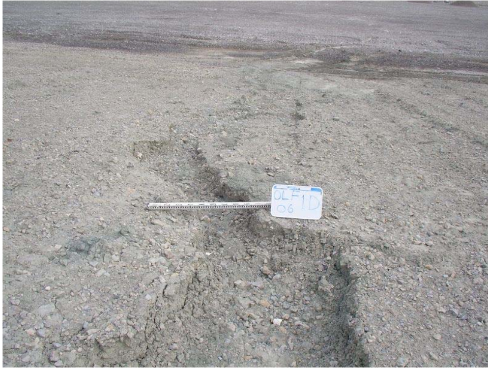
View downslope at waypoint OLF GUL3 - erosion gully is 32 cm deep, as previously measured in 2005.
