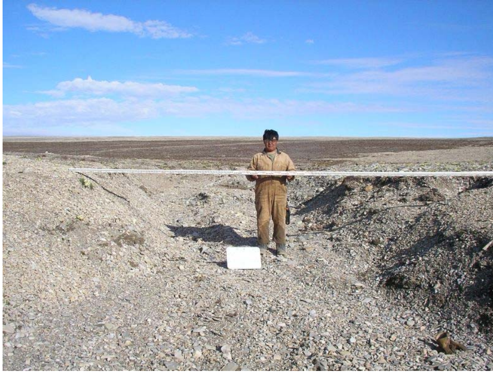
2006 – At waypoint NQG1B. The measured depth of the gully was 1.3 m, which within limits of accuracy, indicate no significant since inspected in 2005.
