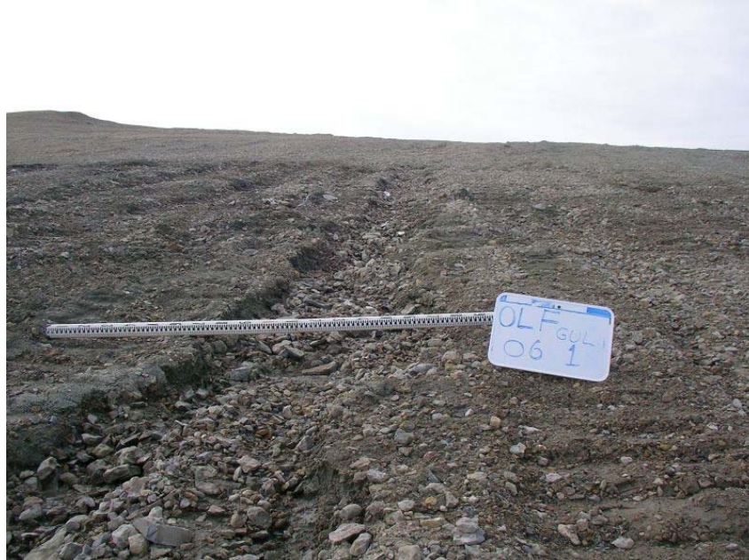
Erosion gully at waypoint OLF GUL1 has a depth of 20 cm and is identical to 2005 observations.
