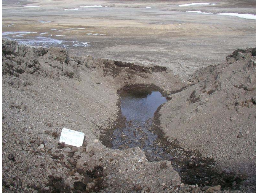
View from waypoint NQ06 20 in middle segment of second erosion gully showing silty sand and gravel, with some cobbles. The water is likely ponded above a frozen horizon.
