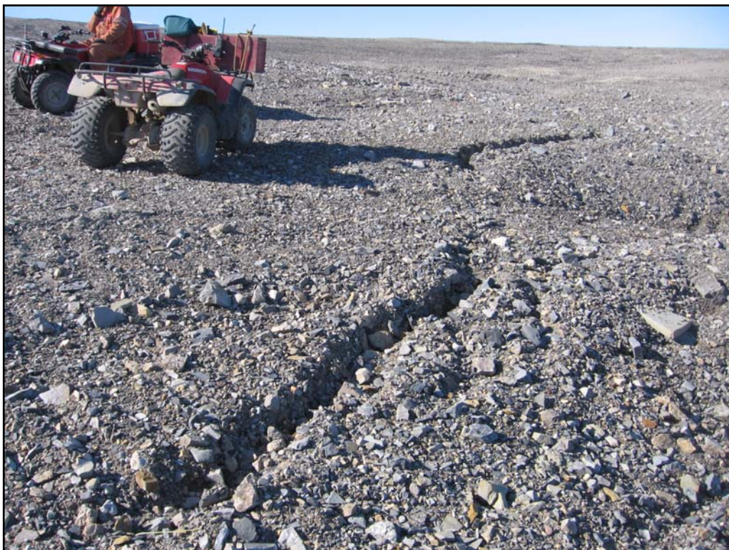
Photo 74- Northing: 8368977 Easting: 558445 Elevation: 18 m. Subsidence area; previously observed tension crack (no change)
