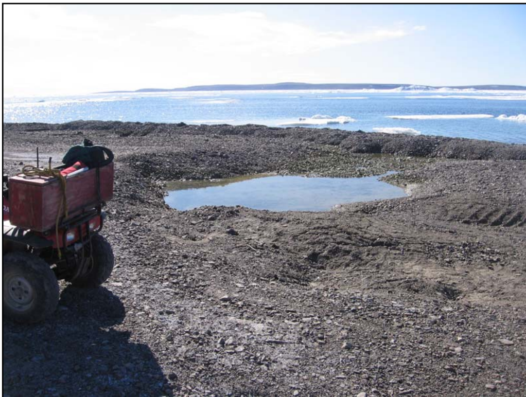
Photo 83- Northing: 8367851 Easting: 557877 Elevation: 4 m. Foreshore; ice thaw settlement
