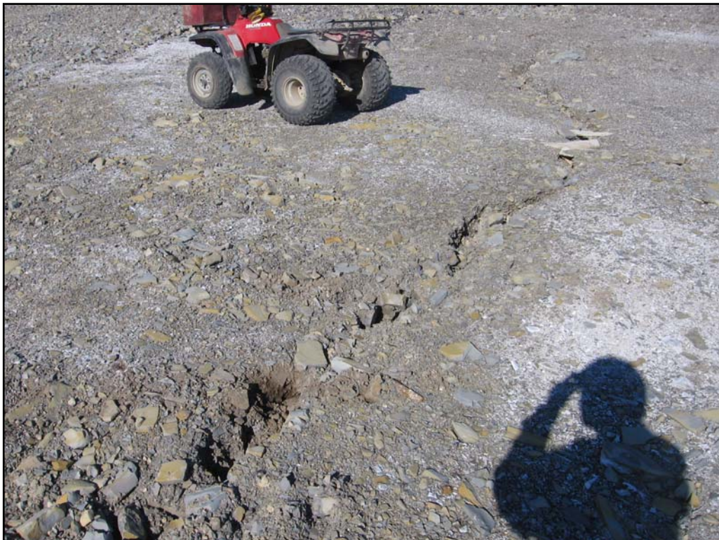
Photo 72- Northing: 8368922 Easting: 558543 Elevation: 25 m. Subsidence area; previously observed tension crack (no change)
