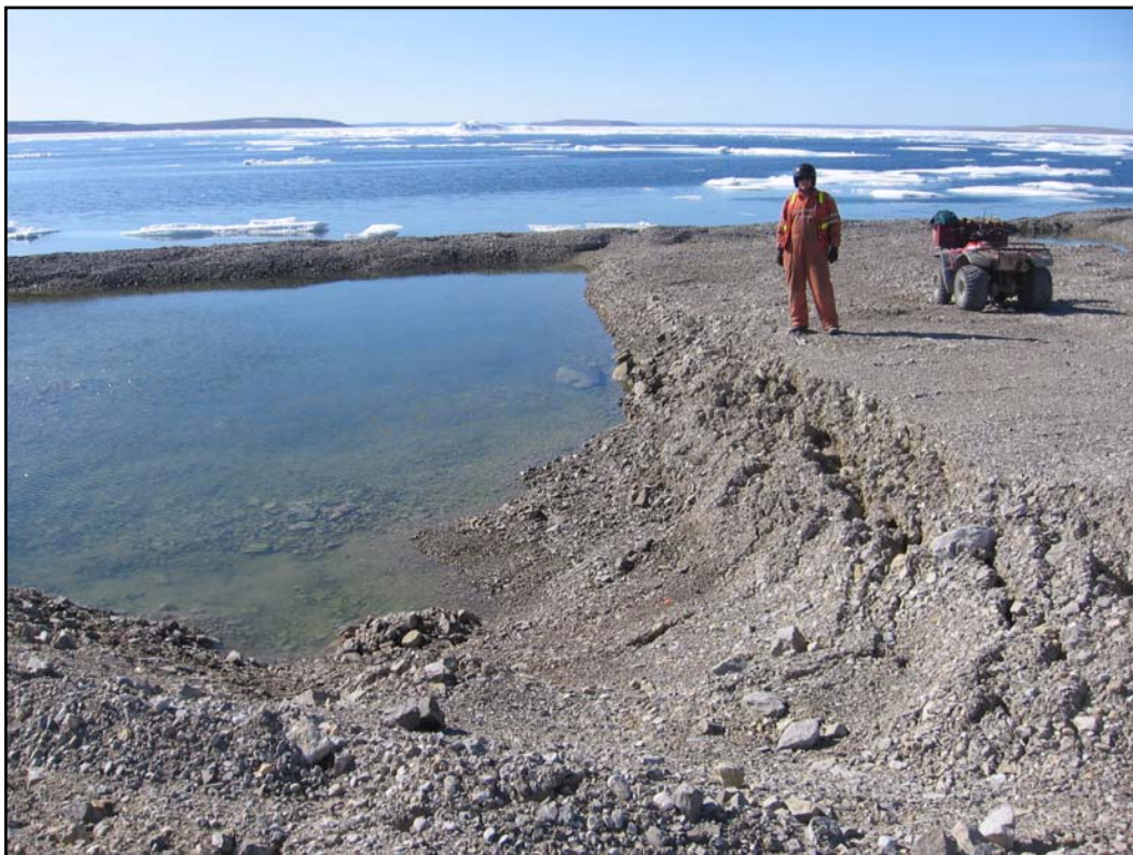
Photo 81- Northing: 8367708 Easting: 557983 Elevation: 3 m. Foreshore; large ice thaw settlement
