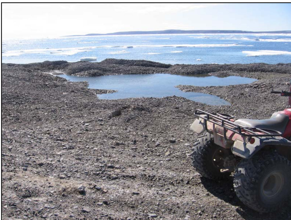
Photo 82- Northing: 8367758 Easting: 557943 Elevation: 6 m. Foreshore; ice thaw settlement
