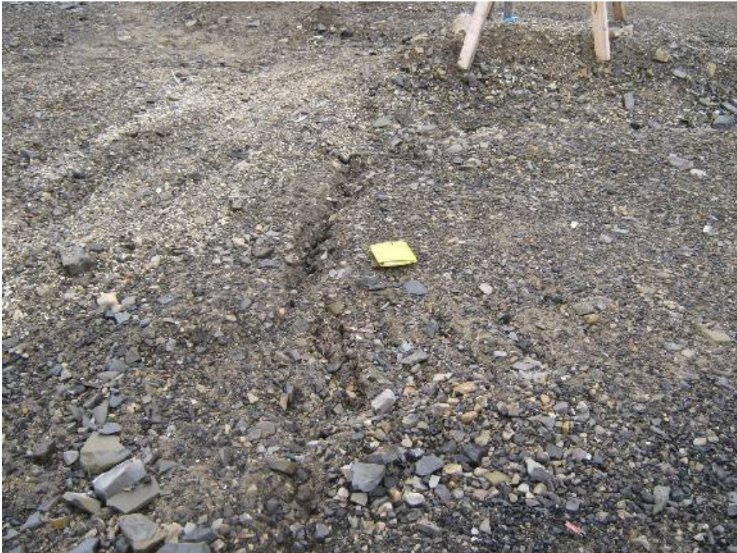
Photo 50- Northing 558515 Easting 8368992 Elevation 17 m Subsidence Area: view of tension crack near bench mark
