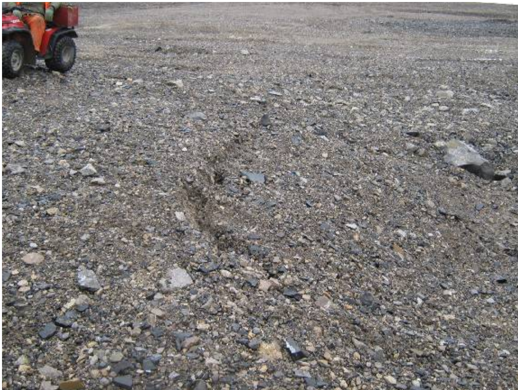
Photo 48- Northing 558447 Easting 8368972 Elevation 13 m Subsidence Area: view of tension crack
