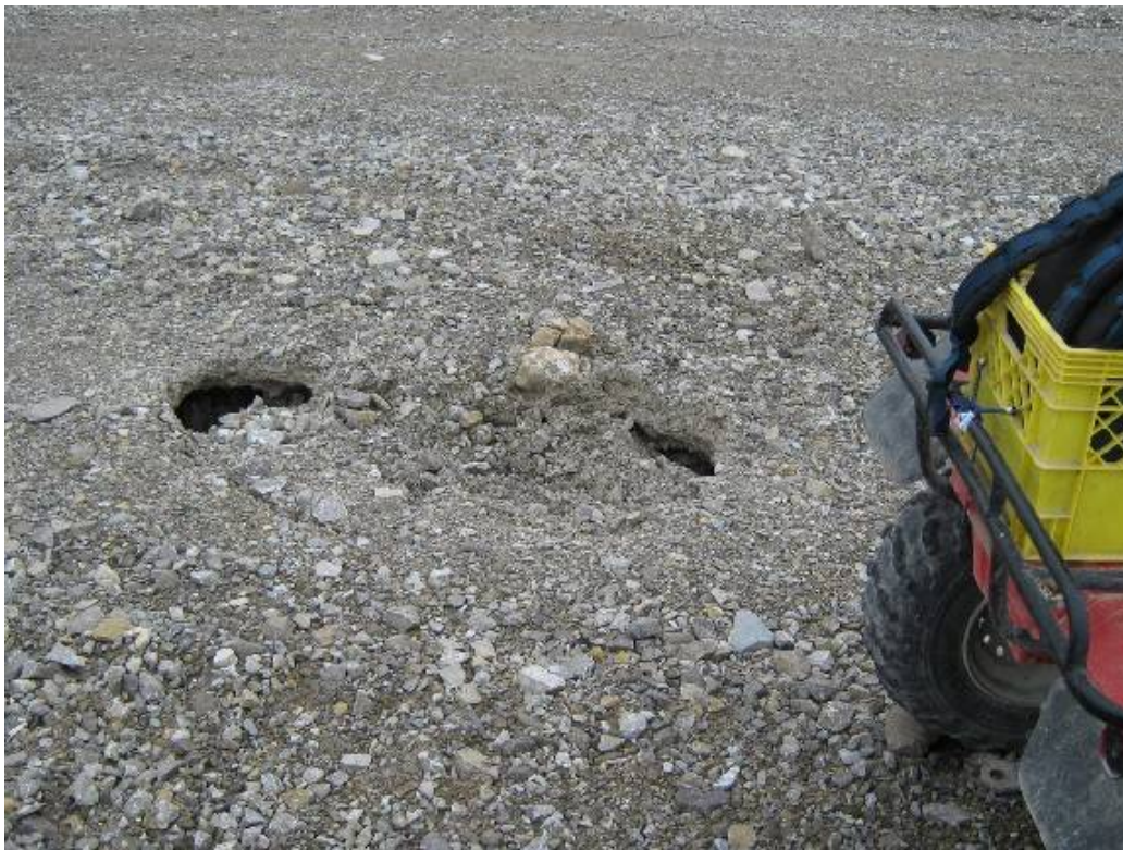
Photo 25- Northing 557983 Easting 8367710 Elevation 8 m Foreshore: 1 m diameter thaw sinkhole about 40 m from shoreline
