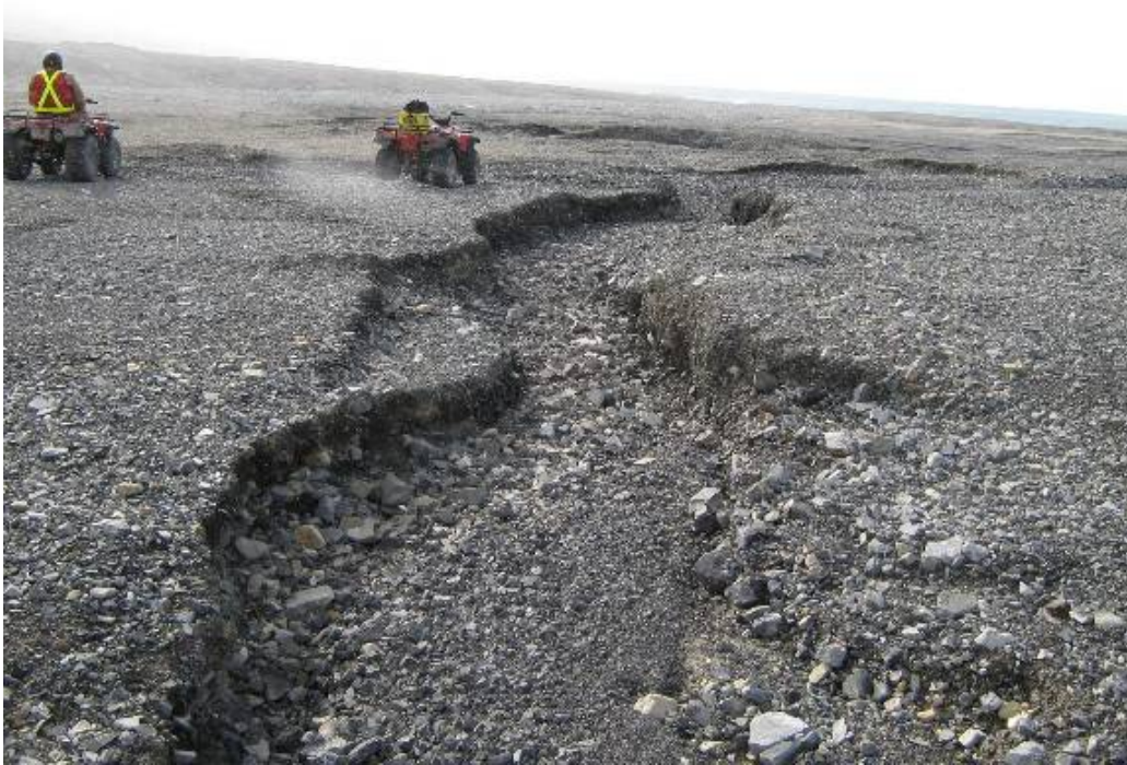
Photo 115- Northing 558779 Easting 8369106 Elevation 9 m New quarry area: erosion gullies meandering over floor of quarry
