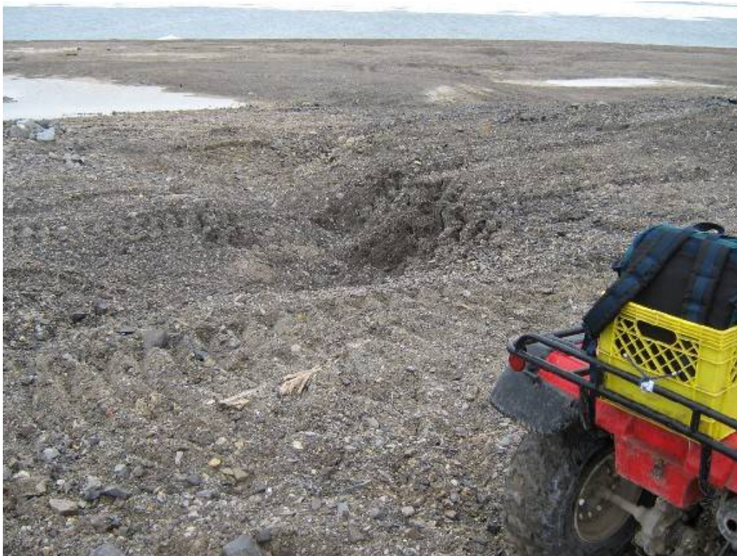
Photo 45- Northing 558151 Easting 8369131 Elevation 12 m Subsidence Area: thaw settlement (about 1 m deep and 2 m wide)
