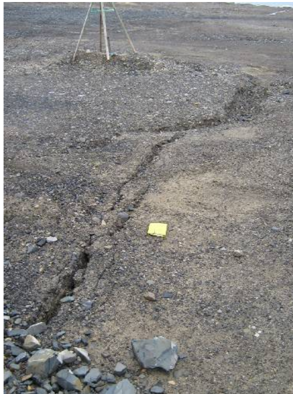
Photo 51- Northing 558515 Easting 8368992 Elevation 17 m Subsidence Area: view of another tension crack near bench mark
