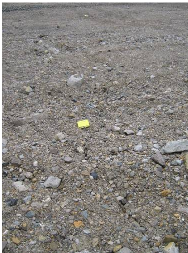
Photo 53- Northing 558576 Easting 8368837 Elevation 28 m View of tension crack upslope of subsidence area
