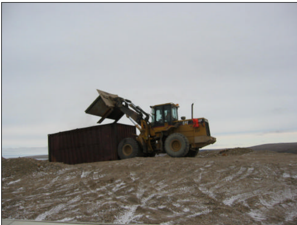
Photo 44 – Front end loader depositing domestic waste into incinerator bin
