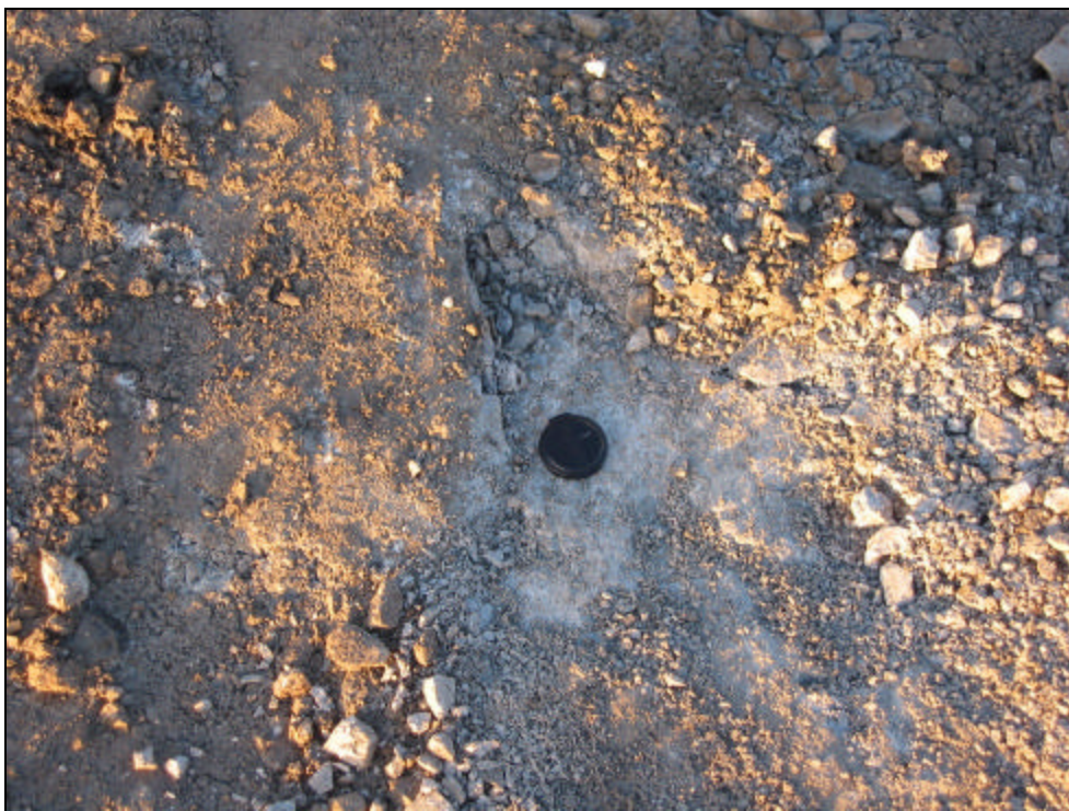
Photo 24 – Fractured limestone bedrock below Concentrate Storage Shed footprint
