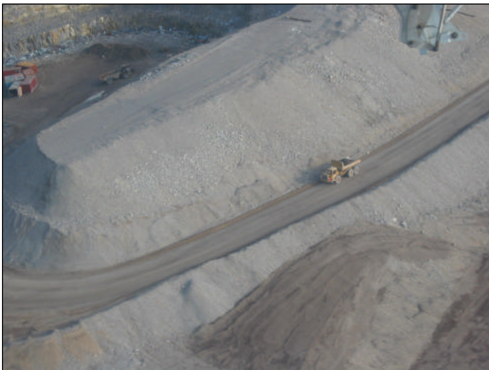
Photo 2 – Aerial view of dump truck transporting contaminated soil for underground deposition via the raise boreholes
