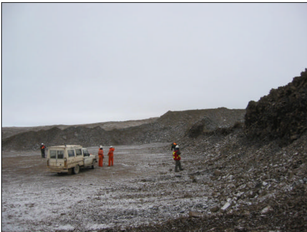
Photo 32 – Inspection group examining New Quarry; the slopes are to be recontoured following final aggregate extraction
