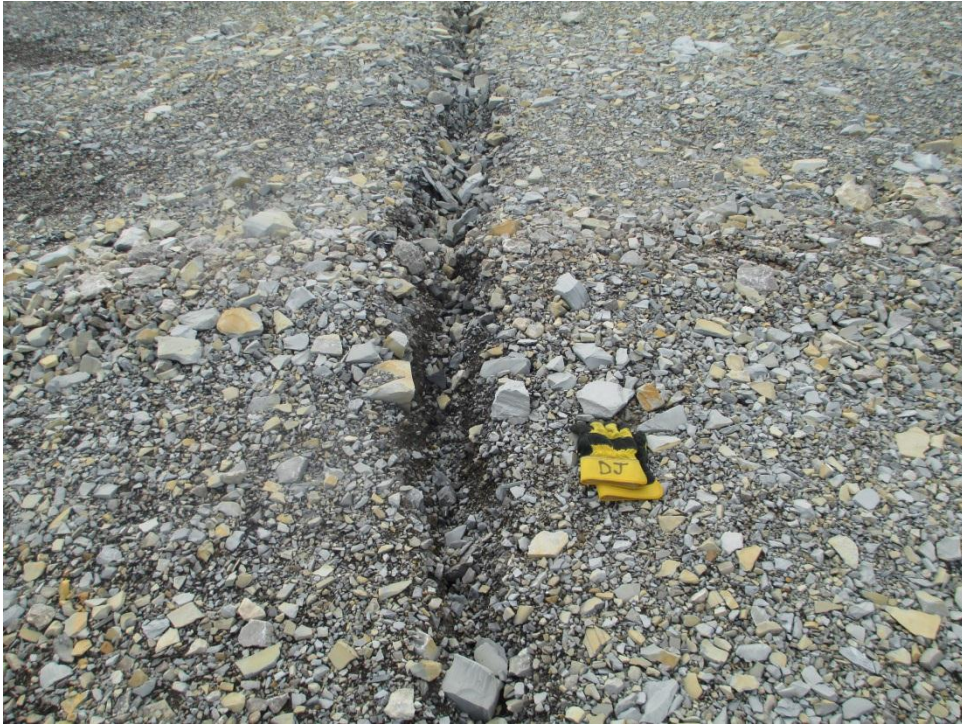
Photo 71, Subsidence Area, old tension crack (WP#60)
