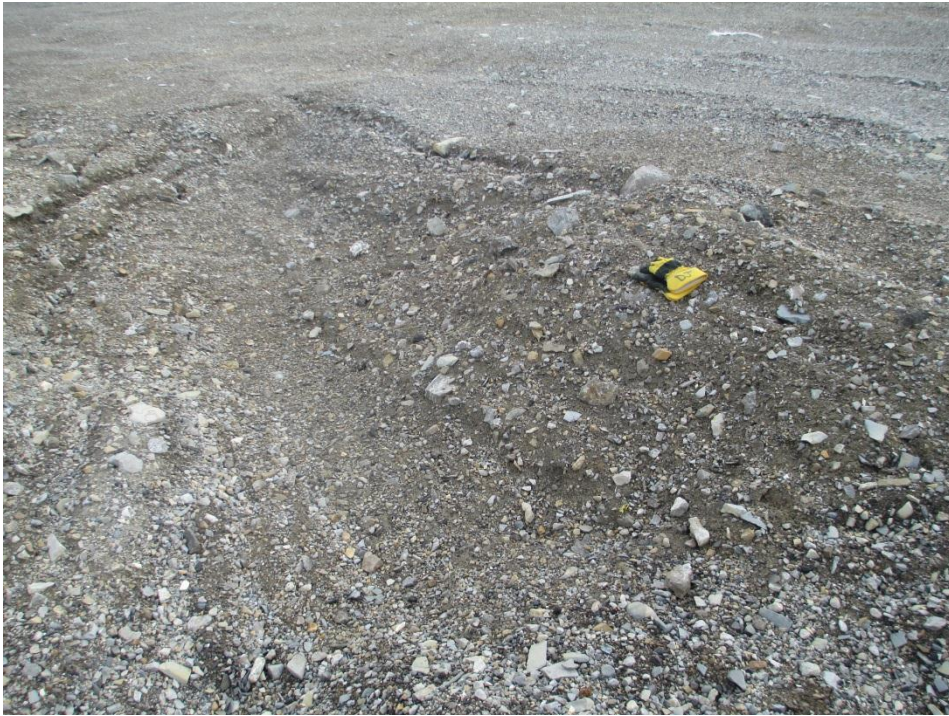
Photo 7, Subsidence Area, thaw settlement area with tension cracks (WP#6)
