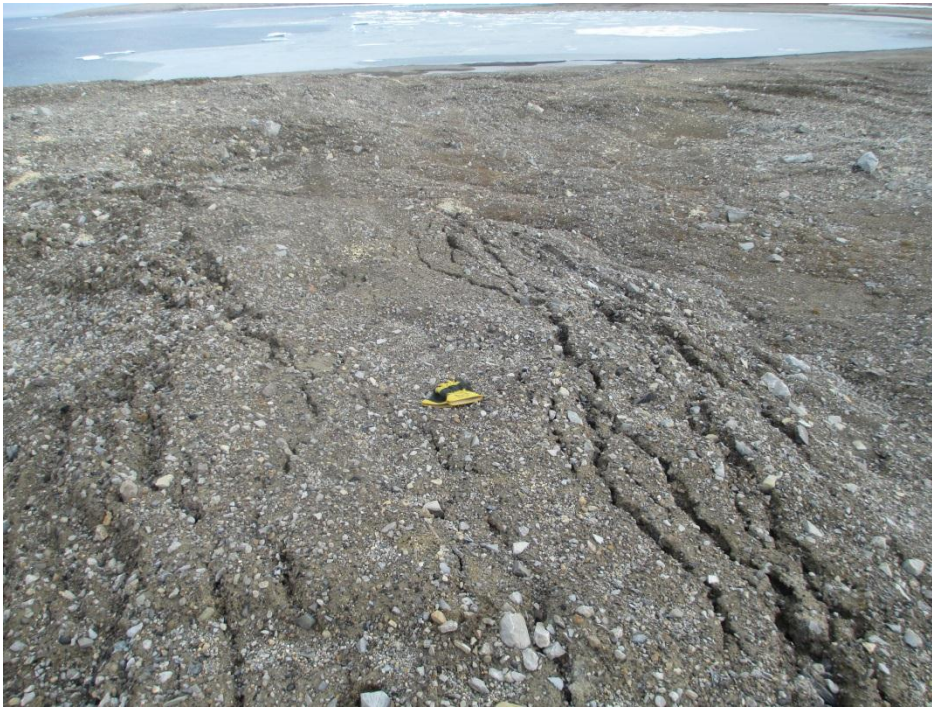
Photo 9, Subsidence Area, tension cracks on slope (WP#8)
