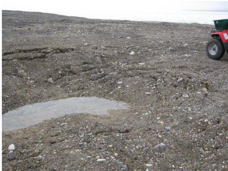
Photo 67, Subsidence Area, Small Thaw Settlement Area (~10m x 10m)
