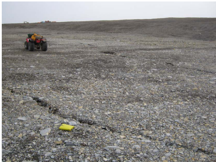
Photo 71, Subsidence Area, Previously Observed Tension Cracks (0.3 m max. width)
