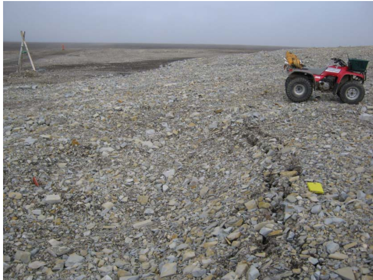
Photo 70, Subsidence Area, Previously Observed Tension Cracks (0.3 m max. width)
