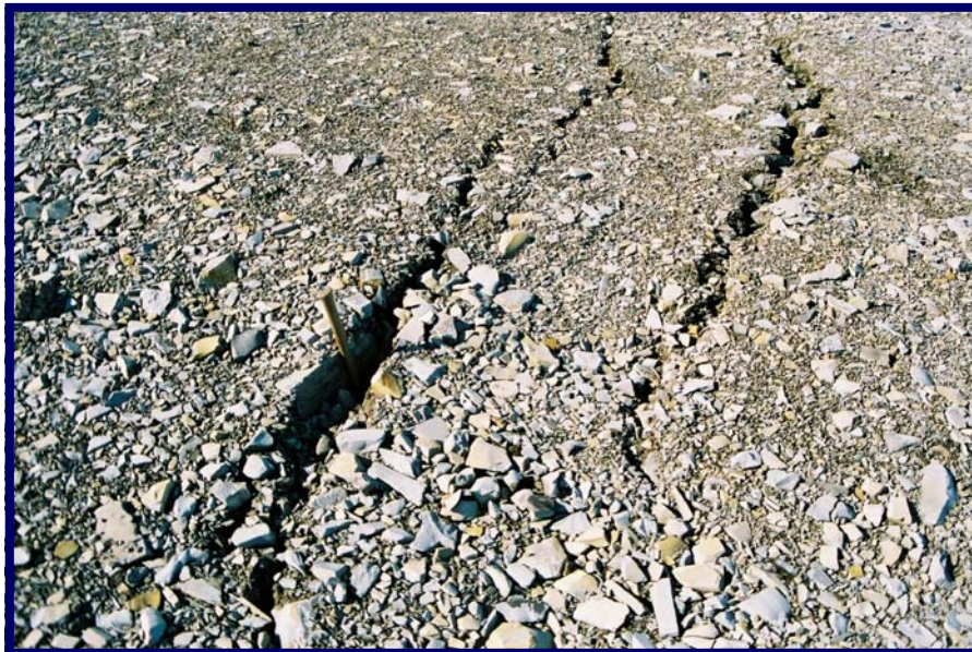
Close-up of cracks in subsidence area. Note rock hammer for scale.
