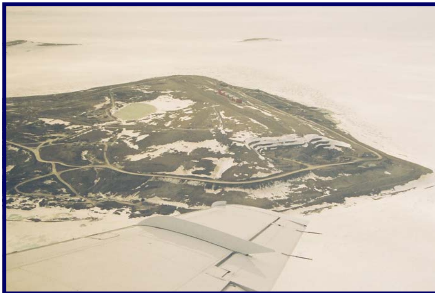
Polaris Mine Site, re-contoured area around subsidence zone and North Portal.
