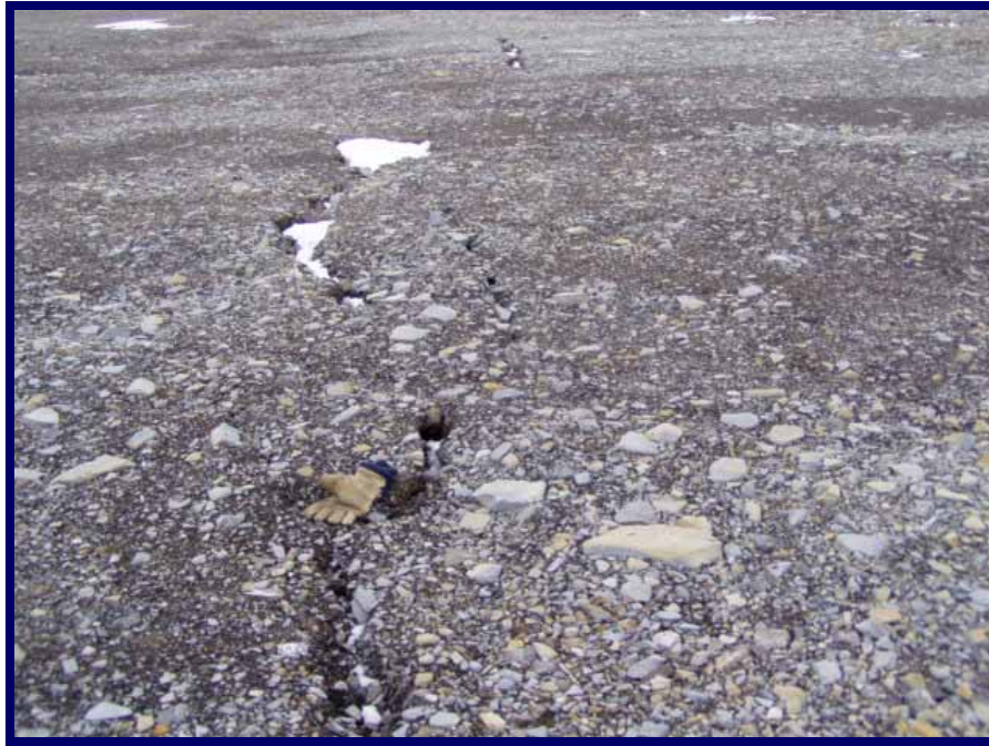
Photo 106: Looking south along one of several large cracks found in subsidence zone. Crack can be traced for several tens of metres. Width varies up to 150 mm and ground is open 10 to 30 cm deep. These have been reported in previous inspections and there is no obvious change. Teck Cominco has now surveyed all these in for record purposes.
