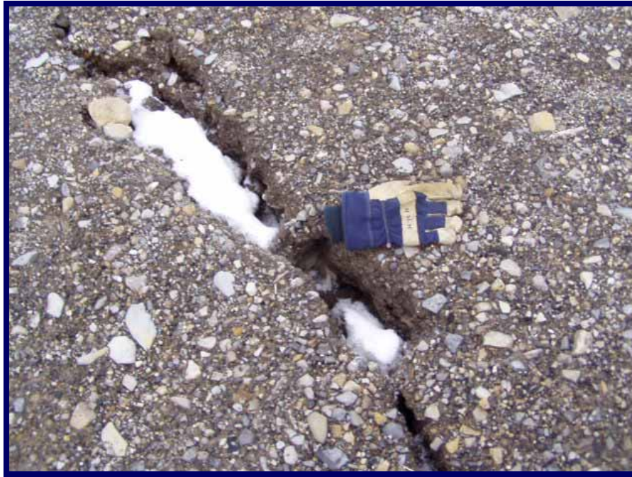
Photo 108: Close up of another snow-filled crack in subsidence zone.
