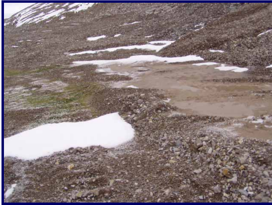
Photo 94: Seepage water coming from slumped material at toe of failure zone.
