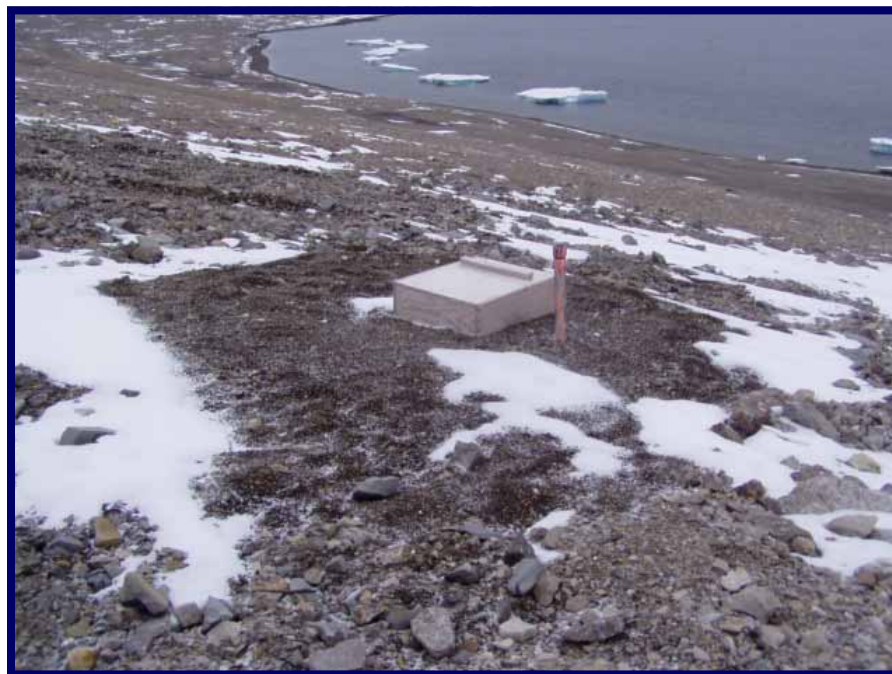
Photo 70: Plywood protective cover for thermistor installation to monitor ground temperatures in landfill cover.
