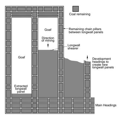
Fig. 1.4 Typical Plan View of a Series of Longwall Panels
