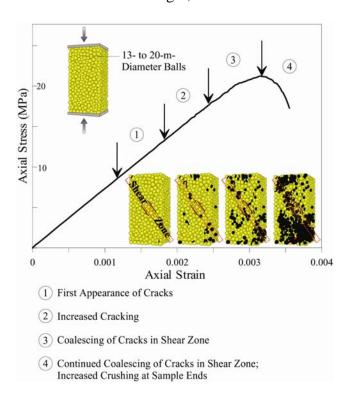
Figure 12. Synthetic Rock Mass Triaxial Test
