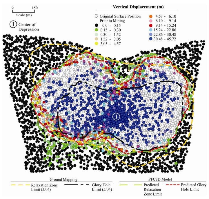
Figure 15. Plan View Map of Surface Movement and Subsidence Limits—Goathill Orebody Model
