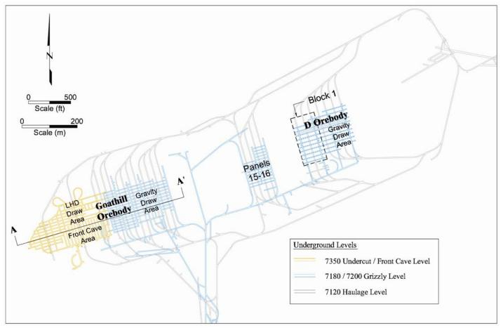
Figure 2. Plan View Mine Layout
