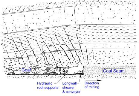
Fig. 1.2 Cross Section of a Typical Longwall Face
