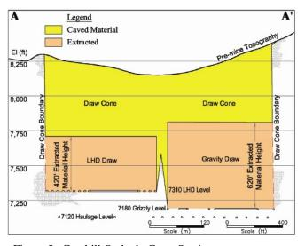
Figure 5. Goathill Orebody Cross Section
