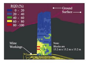
Figure 11. RQD Block Model—D Orebody Block 1
