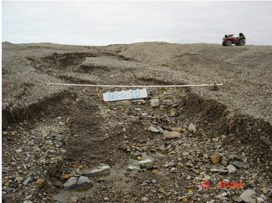
At waypoint NQG1D, depth of gully is 52 cm, and width at base is 3.2 m.
