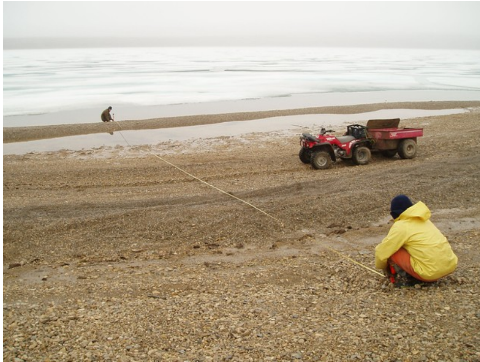
East Quadrant Pin at Station 9 on July 17 2005 – distance to shoreline is 26.7 m.
