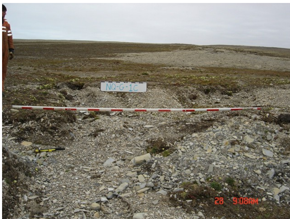
At waypoint NQG1C, depth of gully is 51 cm, and width at base is 3.1 m.
