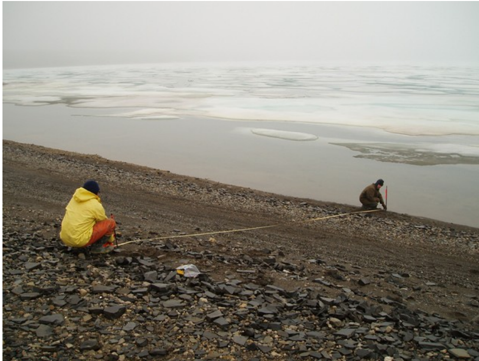
West Quadrant Pin at Station 11 on July 17 2005 – distance to shoreline is 10.3 m.
