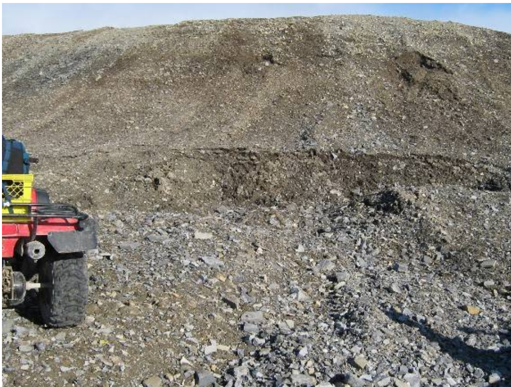
Photo 112- Northing 559102 Easting 8369202 Elevation 15 m New quarry area: settlement area at toe of perimeter slope
