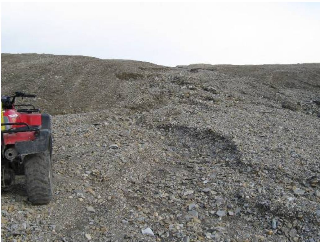
Photo 108- Northing 558880 Easting 8368714 Elevation 25 m New quarry area: self-armouring erosion gully
