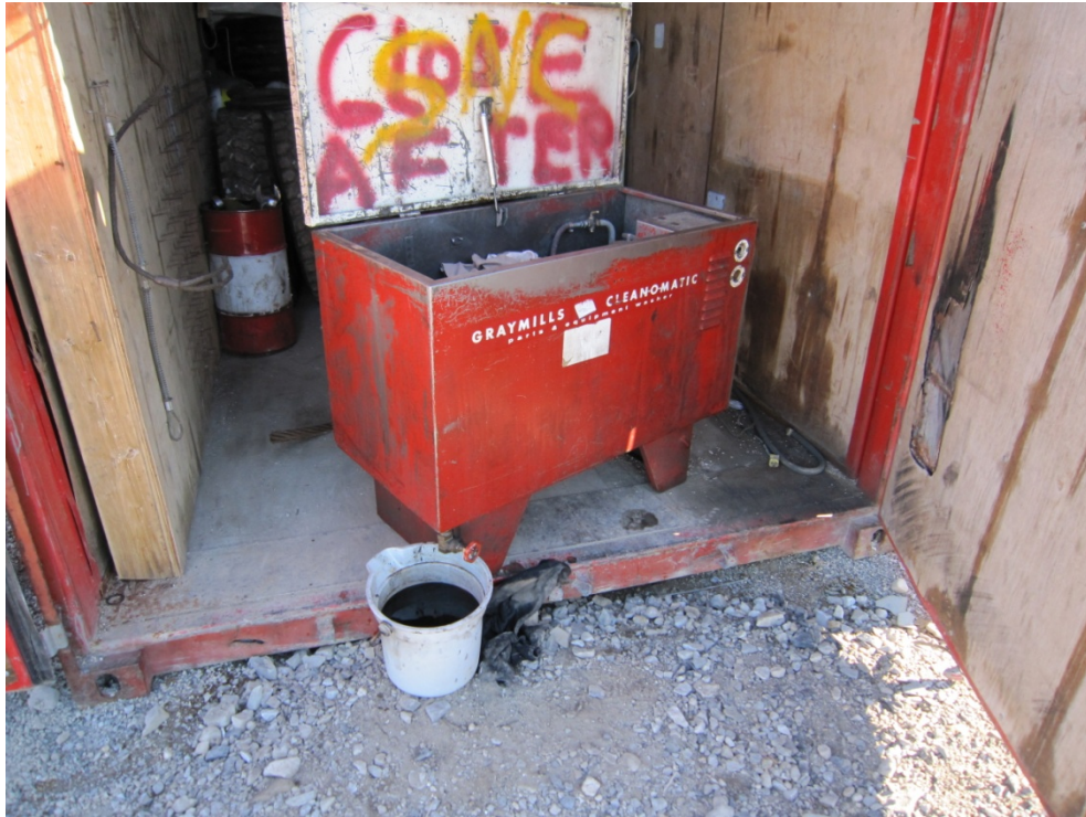
Photo #17 – Draining Parts Washer Reservoir To Prepare It for Shipping
