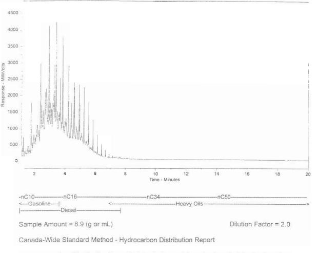
The Hydrocarbon Distribution Report is intended to assist you in characterizing hydrocarbon products that may be present in your sample. The scale at the bottom of the chromatogram indicates the approximate retention times of common petroleum products, and of four n-alkane hydrocarbon marker compounds. Comparison of this report with those of reference standards may also assist in characterizing hydrocarbons present in the sample.
