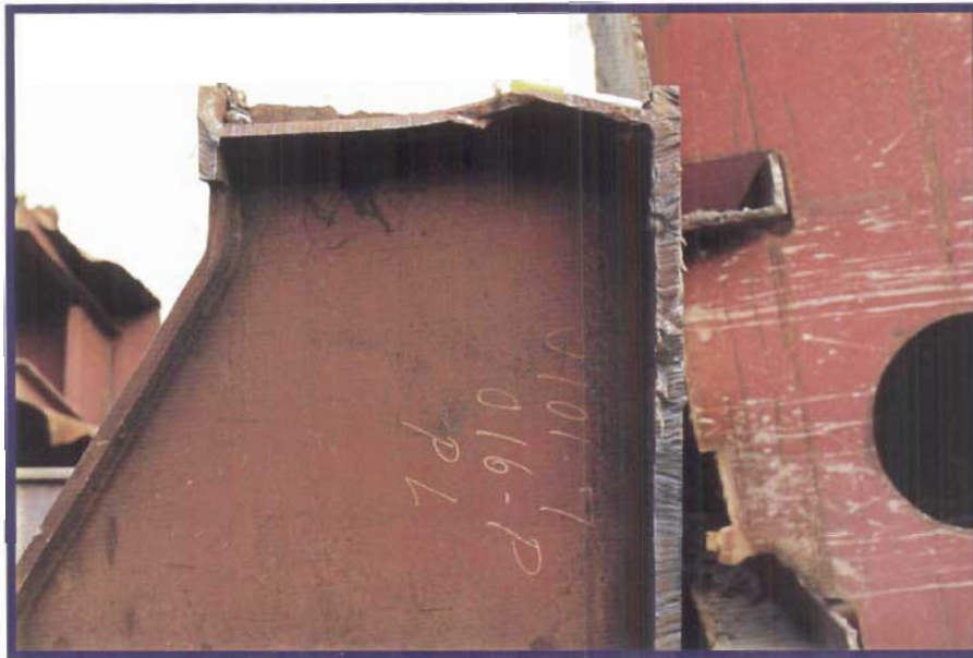
Photo 45 Close up view of cut section of barge hull. (Note pen for scale).
