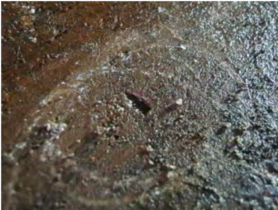
Photo 1756: Pit at bottom plate – repair welded.
