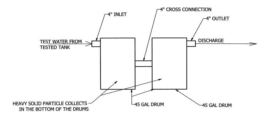
TEST WATER SOLID PARTICLE COLLECTOR
