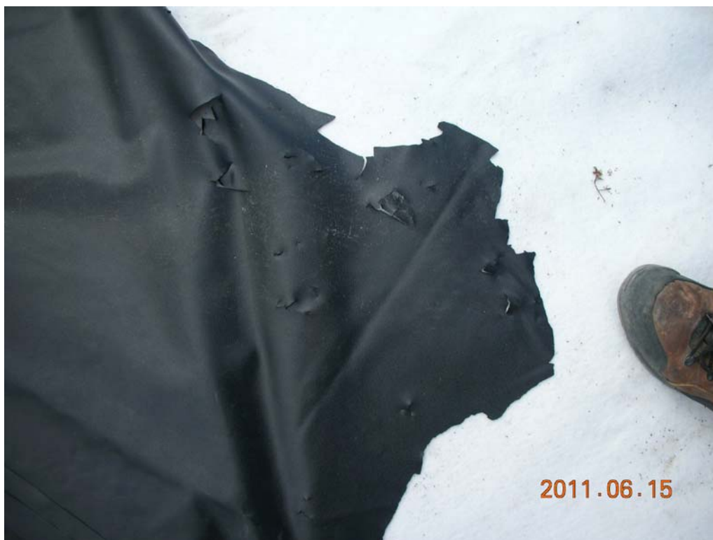
PICTURE 4: Lagoon Liner with Evidence of Polar Bear Teeth Marks
