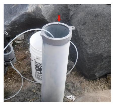
Photo 5-1: Casing of well MW-06. Locking ring on well casing has split.
