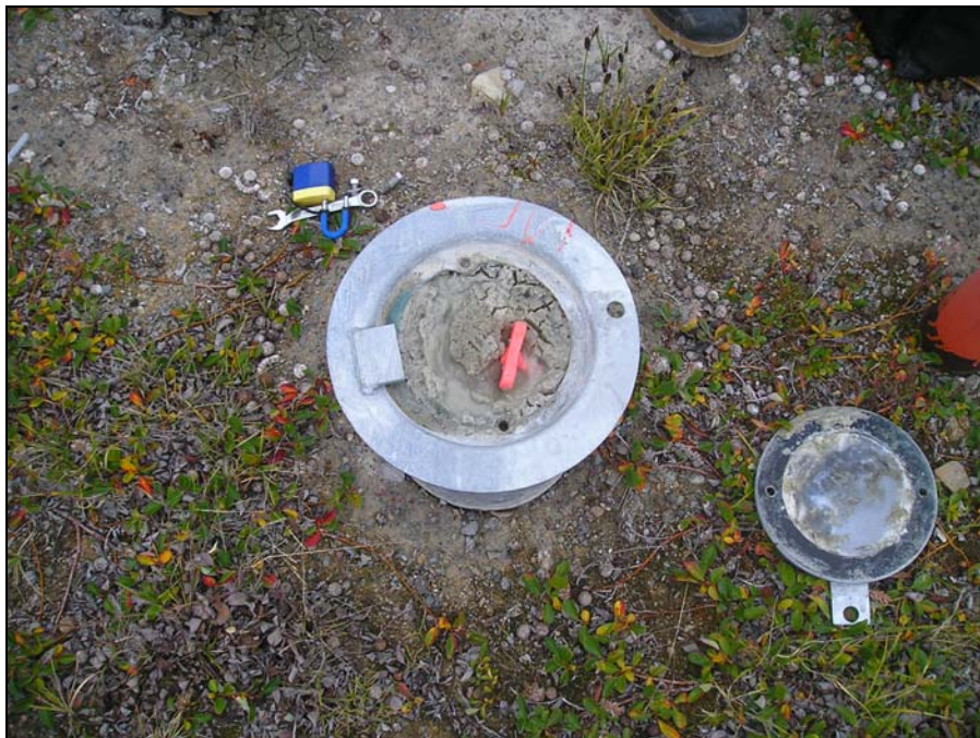
Monitoring well MW-9 (Upgradient). Sample CM-MW-9 collected. Bentonite swollen over TOP.
