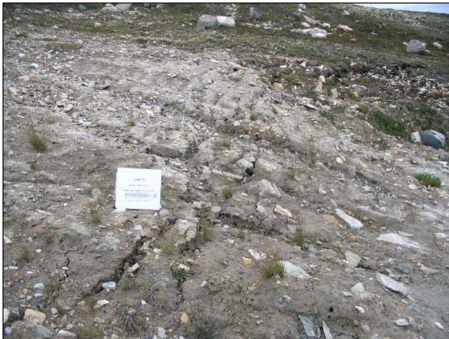
Photo WLF-8B, Easting: 494491, Northing: 7668172, Direction: 270° West Landfill; tension cracks above thaw settlement area, maximum width 5 cm, maximum observed depth about 20 cm. Scale: photo placard dimensions are 29.4 cm wide by 27.5 cm in height.
