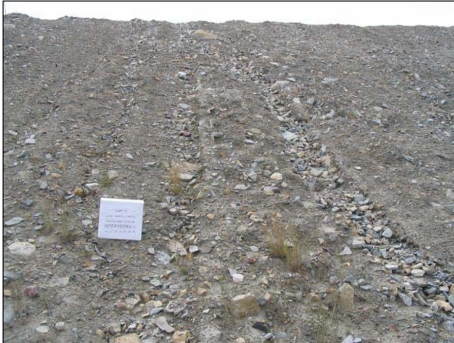
Photo MLFN-9, Easting: 495898, Northing: 7667542, Direction: 200° Main Landfill North; view of erosion gullies Scale: photo placard dimensions are 29.4 cm wide by 27.5 cm in height
