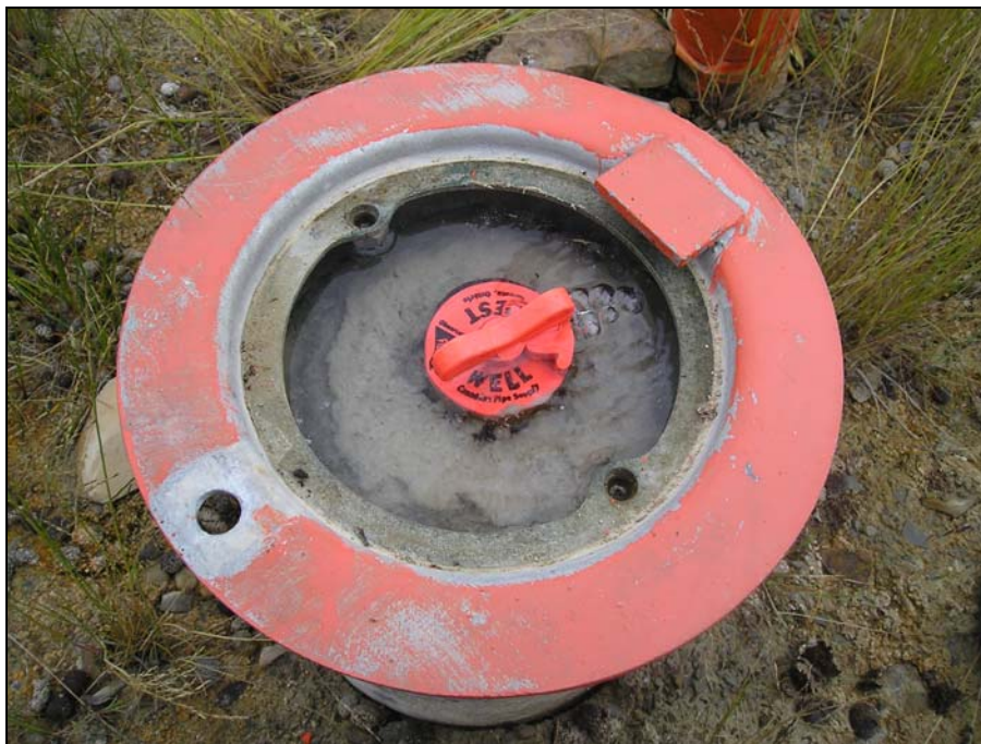
Monitoring well MW-7. Sample CM-MW-7 collected. Bentonite swollen to top of pipe (TOP) and standing water inside well casing over TOP.
