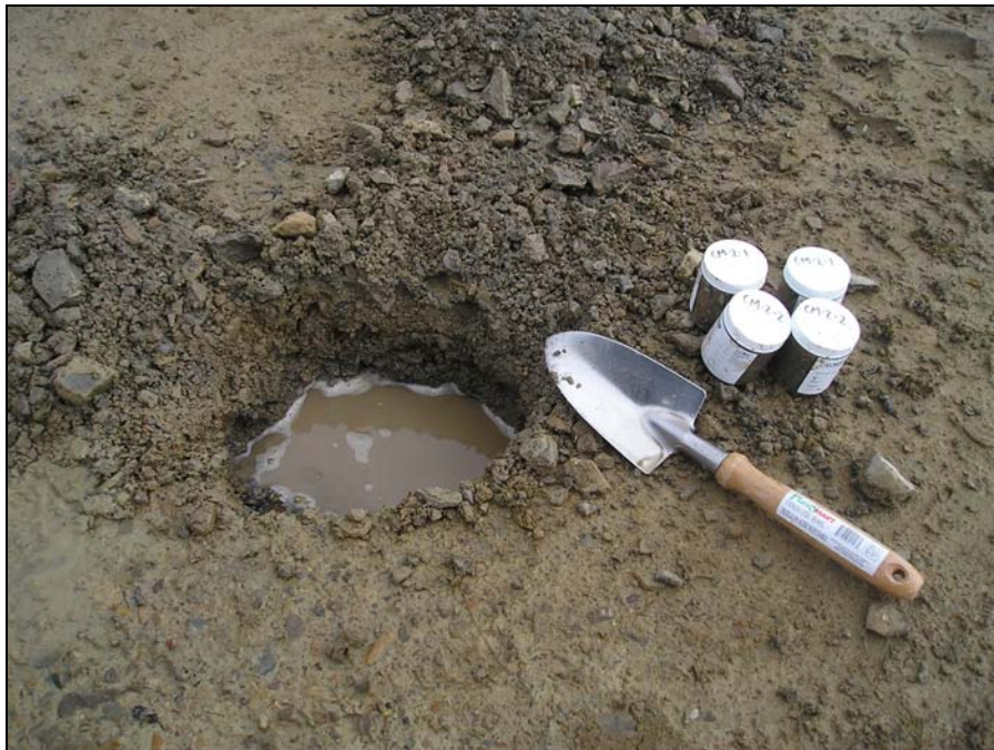
Test pit CM-2. Samples CM-2-1 and CM-2-2 collected. Water table reached at 20cm.
