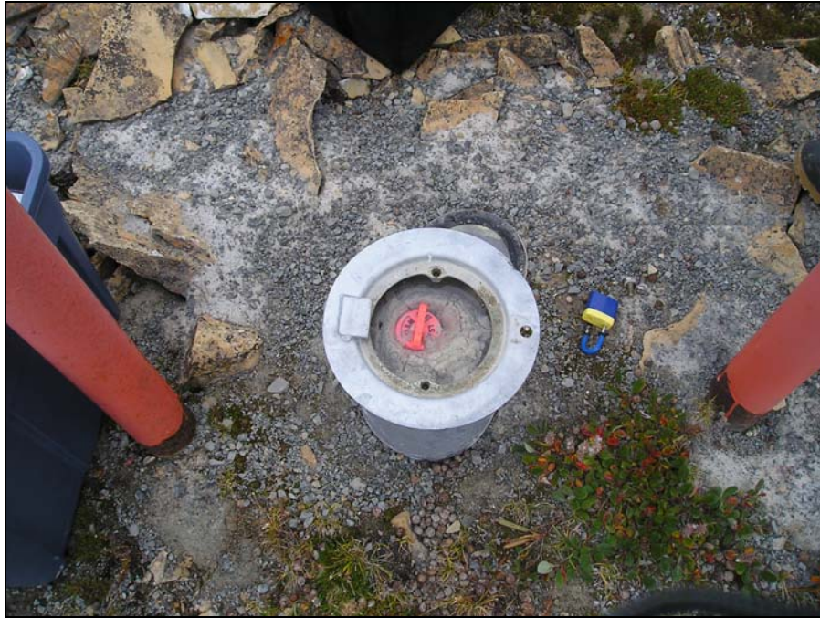
Monitoring well MW-3. Sample CM-MW-3 collected. Bentonite swollen to top of pipe (TOP) and standing water inside well casing over TOP.
