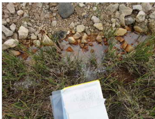
SBLF-15: (left) View northwest at staining in ponded area on southwest corner (10 m L, 0.2-1 m W) - FEATURE B SBLF-16: (right) View of non-hydrocarbon sheen on water at southwest toe (10 m L, 0.2-1 m W) - FEATURE B
