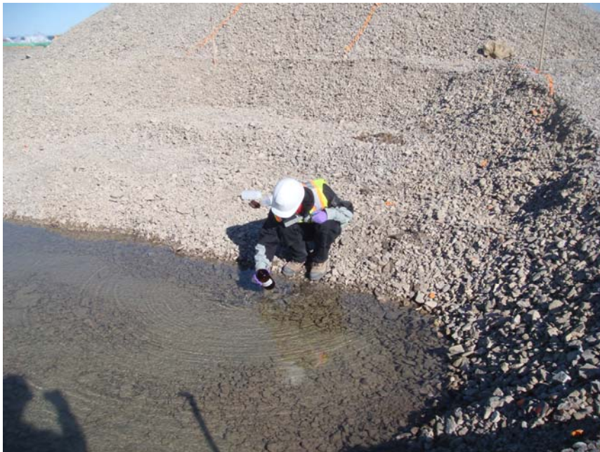
Photo 2 (DSCO3463) Sample 10-05255 Pin-2 Sampling water collected at Lobe N excavation at the Airstrip Landfill.
