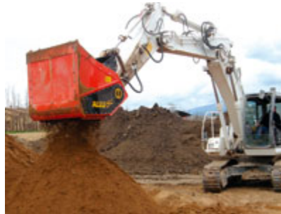
Figure 1 Typical Allu bucket attached to an excavator
