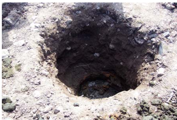
Photo 14. Hole through till cover to tailings beneath consisting of approximately 90 cm of till overlying 30 cm of unfrozen tailings (predominantly B zone tailings with thin (~5cm) layer of Shear zone tailings immediately above frozen layer).
