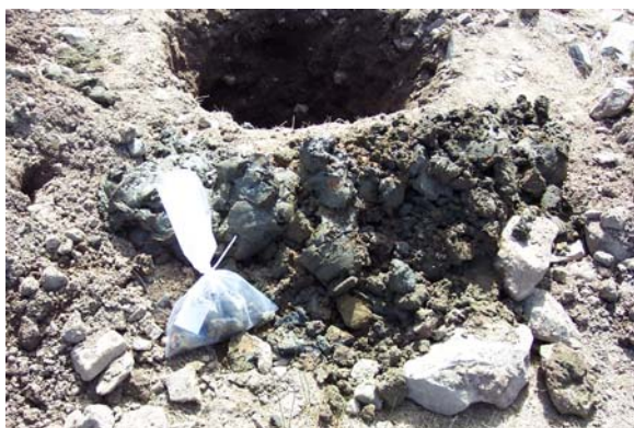
Photo 13. Photo showing tailings excavated from beneath the till cover, predominantly B zone tailings (grey). Tailings sample collected.
