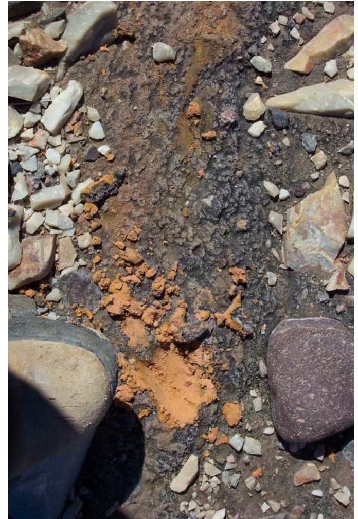
Photo 9 (right). Close-up of exposed tailings – shear zone tailings (orange) with blackened surface coating. Tailings sample collected.
