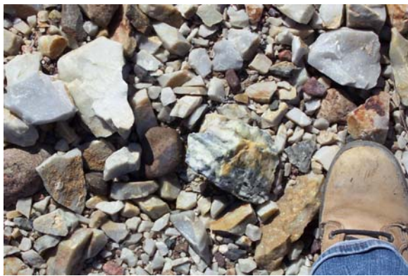
Photo 2. Typical composition of north end of dam construction material, note sulphide-rich quartzite locally stained.
