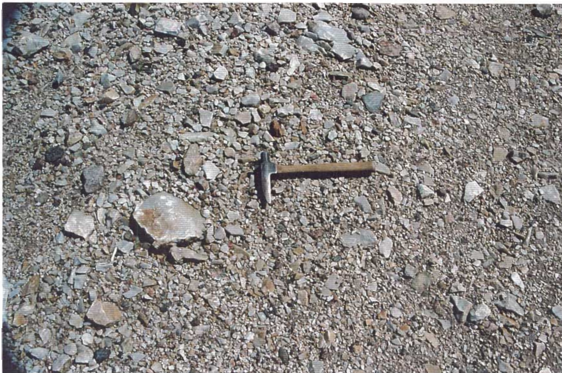
Consistency of typical materials exposed in crest of tailings dike. Mainly quartzite rockfill – well graded from about 30cm to sand size.
