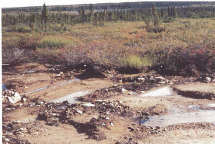
Photo 28. Close up view of the base area where the old waste rock was stockpiled. Notice the dark colour peat layer above the native soil.
