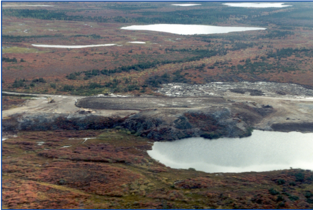
PHOTO 3: Aerial view of the completed capped Shear Lake waste rock pile. Shear Lake is visible in the lower right corner. The original site of the waste rock pile is located across the road from the capped pile. View to the east.
