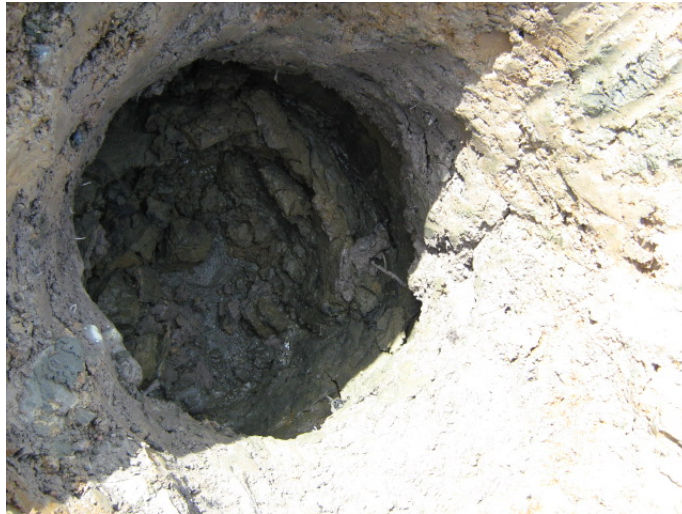
Test pit excavated at T4 on August 5, 2009, showing till cover / saturated tailings interface.
