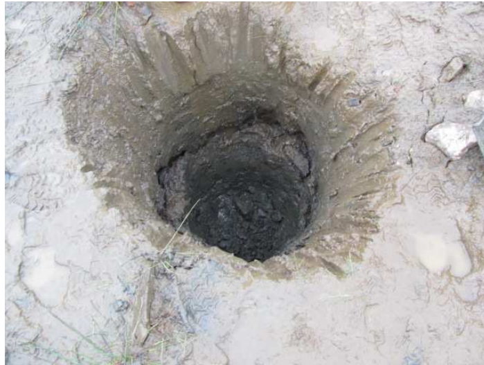
Test pit excavated at T4 on August 4, 2011, showing till cover / saturated tailings interface.
